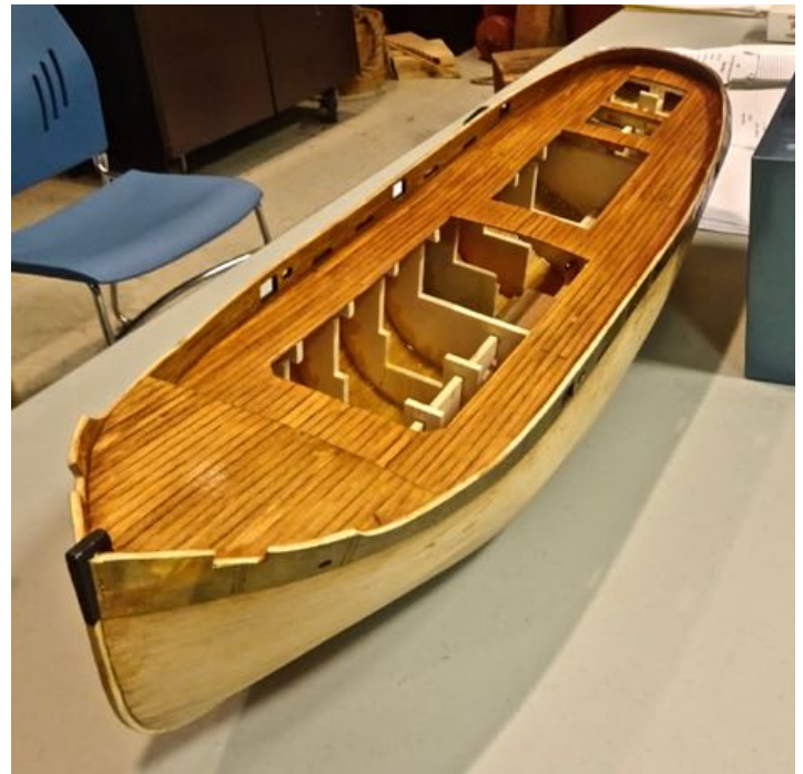
ANTEO 1981 Panart kit. Scale 1:30 Pre-WWII Italian Tug Boat. Lime-wood planking on frame. The interior is coated with slow drying epoxy. Of special note is the upper deck featuring brass bulkheads attached with 200 brass rivets. The model will be radio controlled.
