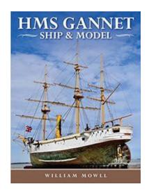
HMSS Gannet was a Royal Navy Dotterel-Class screw sloop launch in 1878 of composite construction with wooden hulls over an iron frame. With her white Mediterranean livery and elegant clipper bow, she was the epitome of the colonial gunboat.
