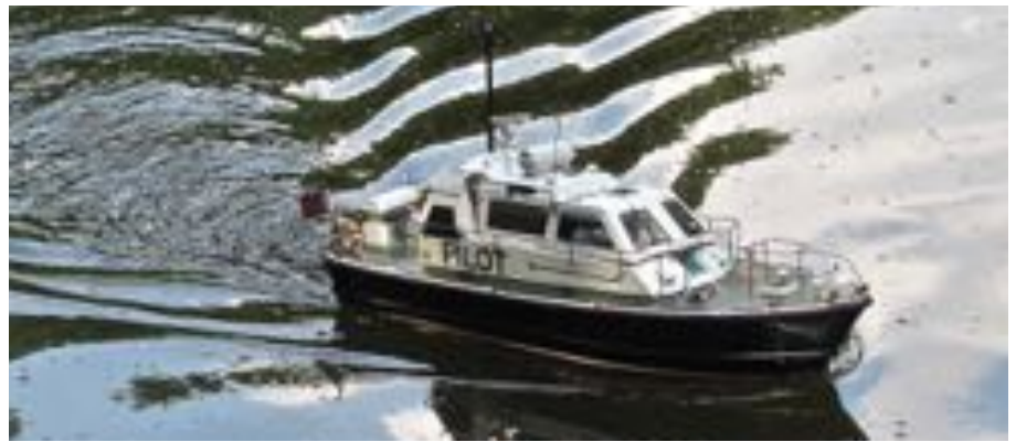
Joe Jordon: "PILOT" BOAT Lesro kit (England) Kit bashed a lot. Wood kit on bulkhead, twin screws.
